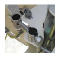
The process is now repeated for the elevation so make sure the elevation locking nuts are loose and start to turn the elevation adjusting bolt in one direction ... as before, wait until the pitch of the beep-beep drops and then stop turning. Start turning the other way listen for the pitch getting higher and then when it starts to drop, stop turning.
